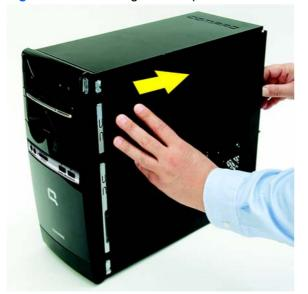
Figure 2-2 Removing the Computer Access Panel
